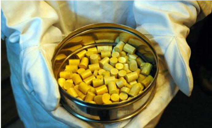
Thorium pellets at BARC (Photo: Pallava Bagla)
